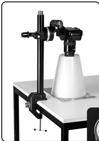
Shooting setup with small cone DUPLI . The camera is supported by table clamp stand ASNEO with tilting head ASMIO .
