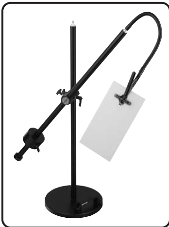
Articulated 360° connector COGEU gives the swivel arm great, continuous mobility. Sliding weight CEGOU counterbalances even heavy loads. Safety ring CEGEE 25 , at the end of the COMBITUBE, prevents the weight from sliding off accidentally.
