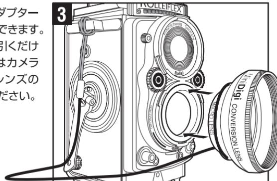
Wipe dust and dirt off the MiniDigi taking lens. Peel cover of the double-face tape off the Adapter Ring supplied as a standard accessory and push it into the taking lens to attach it.
