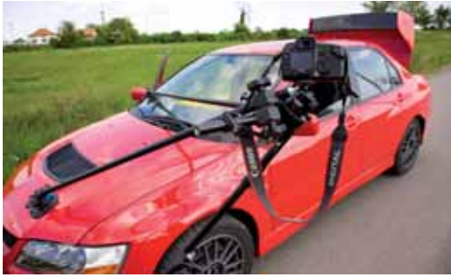
Shooting of a car in motion: COMBITUBE* elements, sucking cups, mini tripod ASNIO and ball head SUPERBALL M-2.
