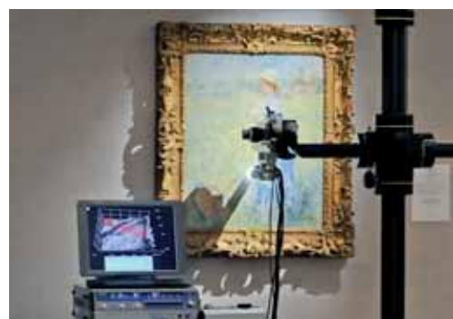
Analysis of a drawing under a microscope: comfortable and efficient way of working thanks to the stable and precise studio stand.
