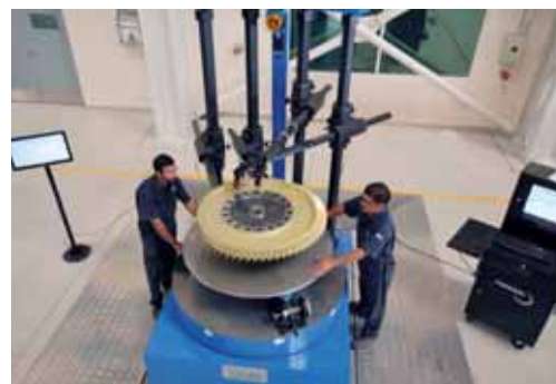
Tactile inspection of the imbalance of high-precision components: four studio stands act as a stable holder for the sensitive sensors.
